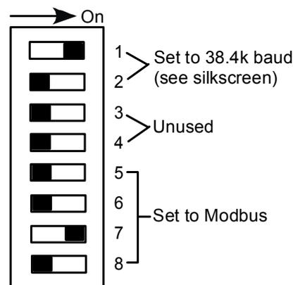
Figure 7. DIP switches set to 38.4k bps and Modbus
