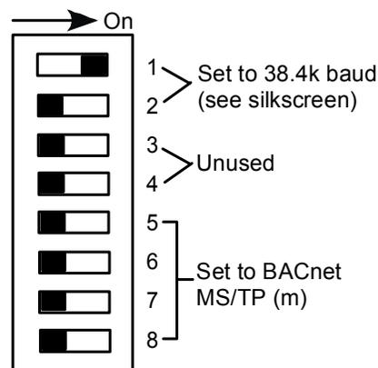
Figure 6. DIP switches set to 38.4k bps and BACnet MS/TP
