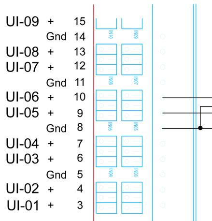
Figure 9. Wiring thermistors
